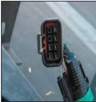
Chassis harness side part number 897364-5300
