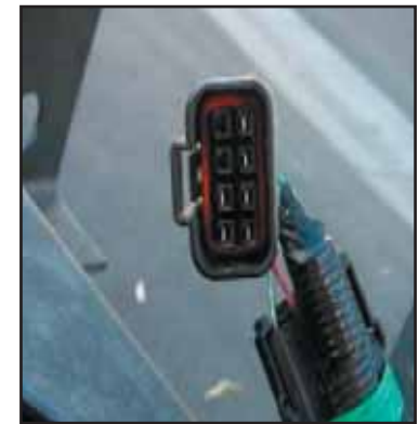
Chassis harness side part number 897364-5300
