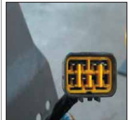
Stop and tail lamp side part number 897364-5310
