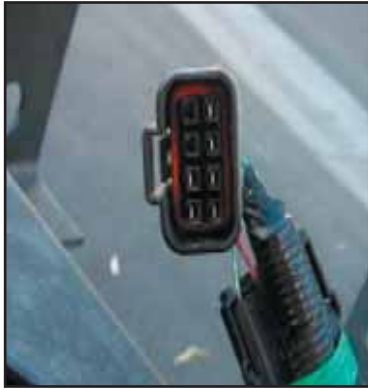
Chassis harness side part number 897364-5300
