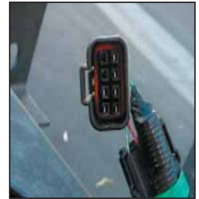
Chassis harness side part number 897364-5300
