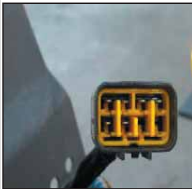
Stop and tail lamp side part number 897364-5310
