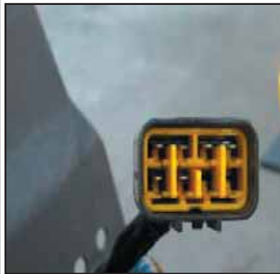
Stop and tail lamp side part number 897364-5310
