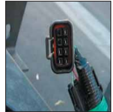
Chassis harness side part number 897364-5300
