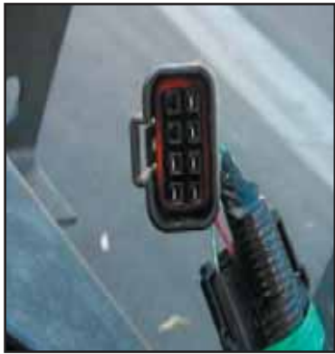
Chassis harness side part number 897364-5300
