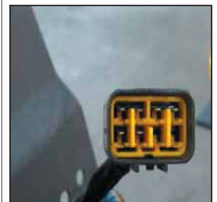
Stop and tail lamp side part number 897364-5310
